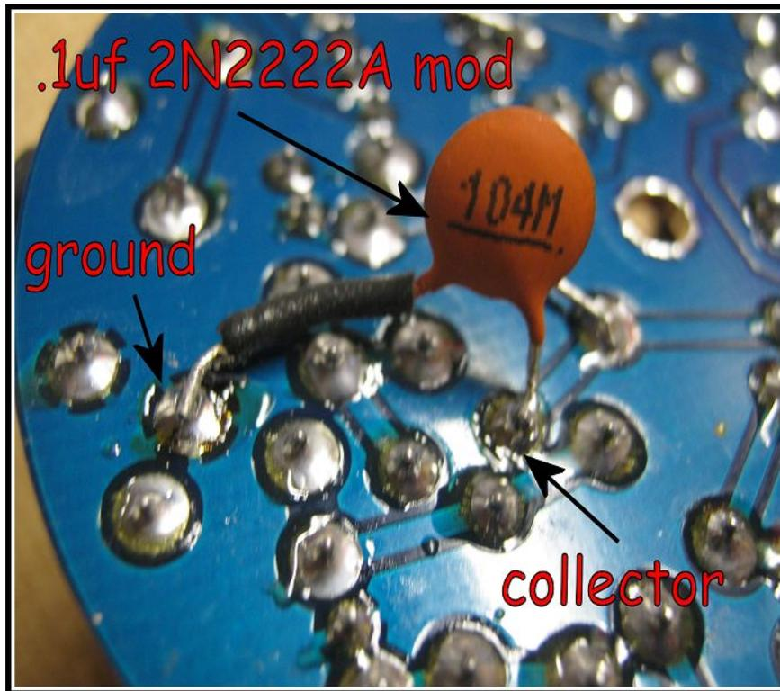
( ) Solder .1uF Cap (104) from Collector of Q1 to ground. You might use a small piece of insulation from a piece of hookup wire or a piece of heat shrink tubing to insulate the cap's long lead heading over to the ground pad.
