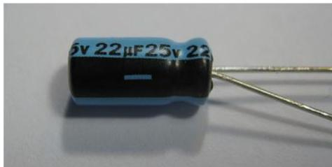
polarized or electrolytic capacitors are either marked similar to non-polarized caps if the body is real small or marked plainly on large body caps
