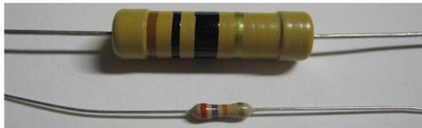
resistors are marked using bands of color which follow a code:
