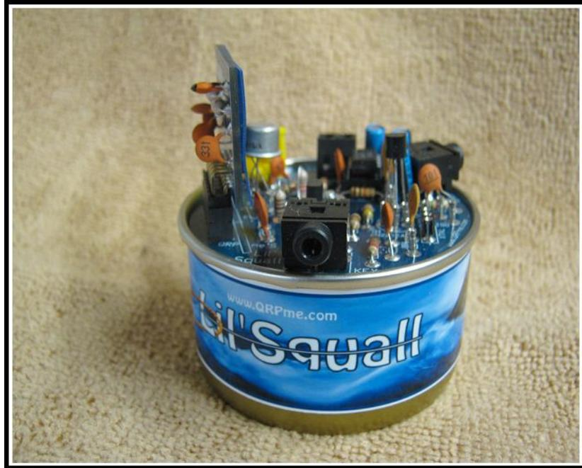
( ) Install board on top rim of the Lil' Squall can using supplied long bolt and nut. **Note:** 10uF Electrolytic Cap Pads closest to the edge of the PCB, at approx. 1 & 2 o'clock, could possibly short to the rim of the can. Use some electrical tape or similar to insulate the pads before installing the board on top of the can.
