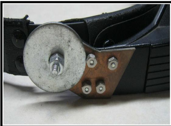
Fender washer & bolt for the hinge and a piece of copper clad pcb stock for a broken side piece and they work as good as they did 30+ years ago!
