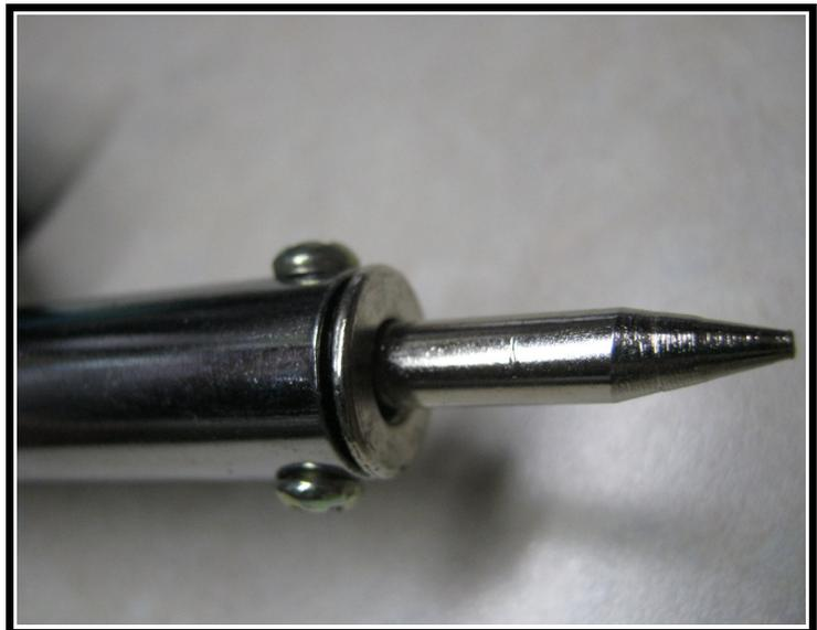
Stay away from this type of iron or use it for either wood burning or plastic melting chores.
