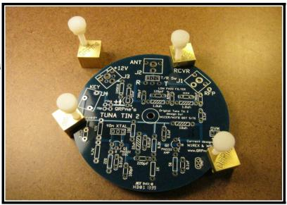
You insert parts on the top side of the board and bend the leads on the bottom side.....like normal.
