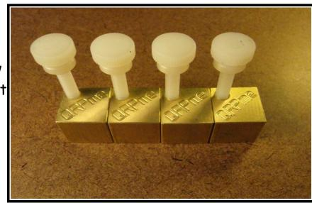
Insert the pcb into the slot at any convienient location on the circuit board and gently tighten the thumbscrew.
