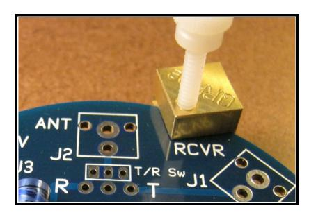
Three clamps work perfectly fine on tuna can boards when they are spead out in a tripod fashion.
