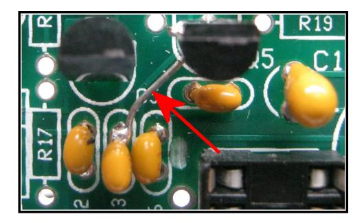
4. When assembling the last stage, install Q2 and C13 first, with about 1/4" of component leads above the board. Then you use a short piece of cut off component lead to make a connection between C13 and Q5 as shown on the schematic. This mod will now cause the oscillator to generate a larger voltage swing on the output signal before it heads on to the signal shaping circuit.
