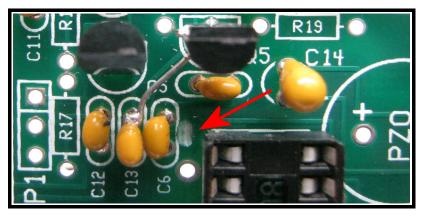
1. Cut the +5V feed to the collector of Q5 where it passes around U1, the Picaxe micro. Just to the left of the DIP socket, the trace passes underneath C6 and then on to the collector of Q5.
