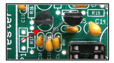
3. The silk screen designator for Q4, the 2N4403 transistor, is backwards. When called for, install Q4 backwards from the silk screen.
