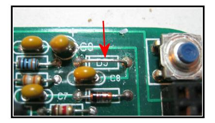
2. D5, a 1N4148 transistor, is not required so install a shorting jumper between the D5 pads instead of a diode.
