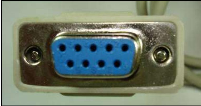
The remote end of the serial cable is cut off and 3 Molex terminal pins are soldered on the Txd, Rxd and Ground (2, 3 and 5 on the PC end) pins. Complete circuit details for both Serial and USB downloading cables can be found at the Picaxe site:
