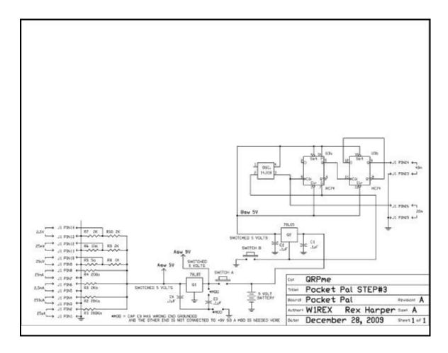
OK. Now we can move on to build the 20m/40m oscillator circuit. You can use the outputs of the oscillator to test frequency counters or receivers etc. Press pushbutton B to power up the oscillator and divide by 2 circuit and the 20m output, 14.31818Mhz, is available on connector pins 25-26 with the ground side of the signal on pin25. The 40m signal, 7.15909Mhz, is available on pins 23-24 with the ground side on pin23.
