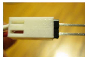
HEADER PULLED BACK INTO HOUSING.
