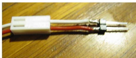
HOUSING 'REVERSED' AS WIRE IS THREADED THROUGH PIN HOLES AND OUT TERMINAL END.
