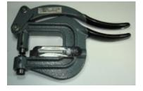
The Harbor Freight deep throat hand punch is a poor man's version of the Whitney Roper Hand punch... BUT IT WORKS!
