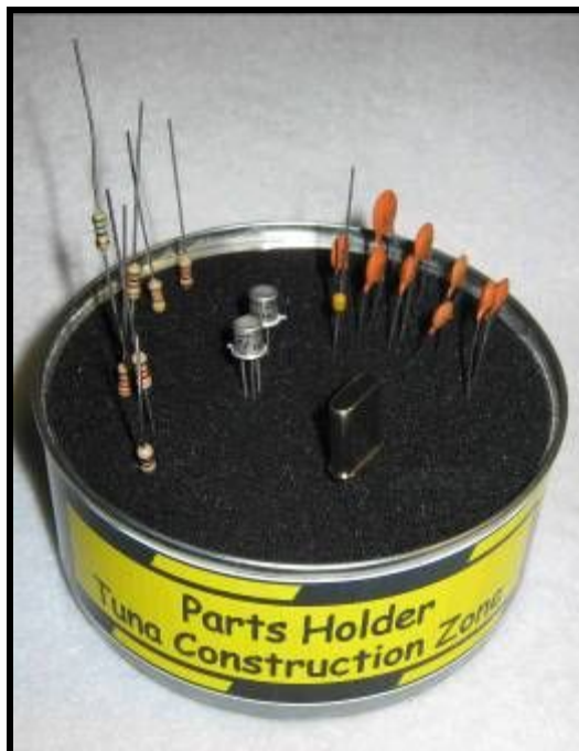
Parts holder made from an empty can and a piece of antistatic foam cut to fit the inside of the can. Cut some corrugated cardboard strips 1" wide, fold many times, and place underneath the foam to lift it up to just under the can lip.
