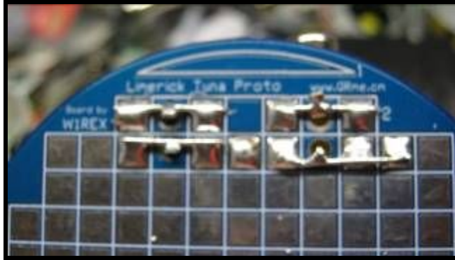
A view of the solder pads for the RCA jack & On/Off switch...
