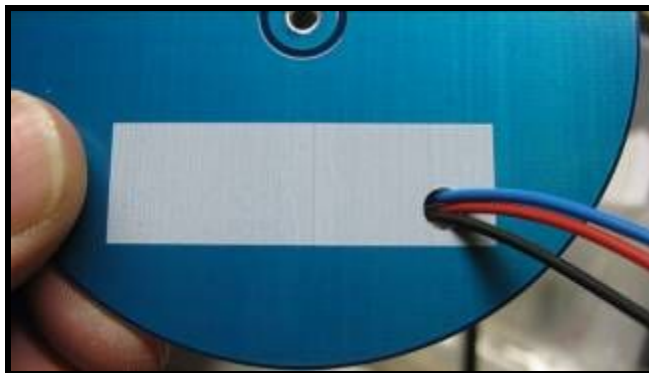
I drilled a hole and passed the fan wires through...
