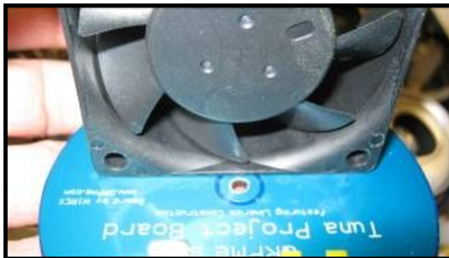
and then Super glued the fan to the board...
