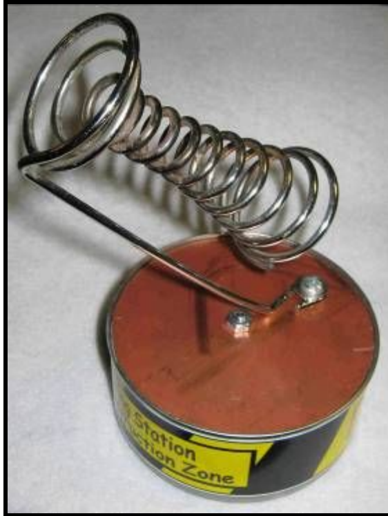
Soldering iron holder made using an old dead soldering station iron holder...
