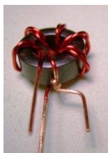
Leads formed ready for installation.
