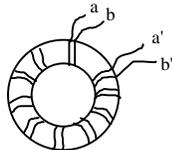
Diagram showing completed bifilar-wound transformer T1. (Note: 10 turns are shown here ... you will need only 6 turns)
