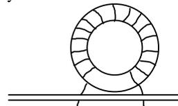
❑ **Constructing transformer T1.** This transformer is a “bifilar-wound” inductor on a toroid core, meaning that you’ll be combining two magnet wires together and winding them at the same time. Measure off a 9” length of red magnet wire, and another 9” length of green magnet wire. These wires should be twisted tightly together as illustrated below.
