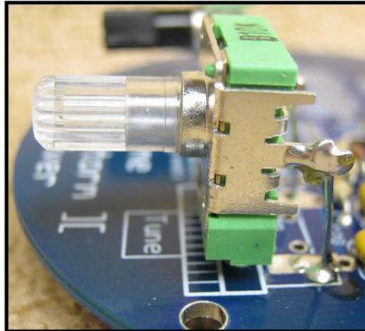
Here is a side view of a Soup-up pot mounted in the wider spaced forward pot pads. The pots are normally mounted flat on the pcb with the shafts perpendicular to the board. In the SS application, you mount them with the shafts parallel to the pcb. Adding short pieces of clipped components leads between the solder tabs and extra grounding holes will add much to the stability of the pot.
