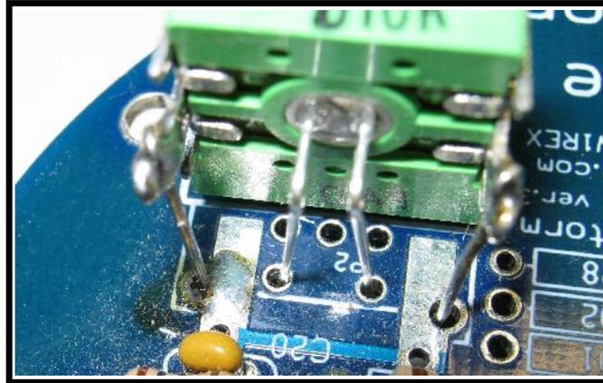
The above picture shows the Soup-up pot with an LED installed into the pot shaft. Note the 2 holes for the LED leads. Installation of the pot and LED is the same for either the Gain or Tune pot & LED.
