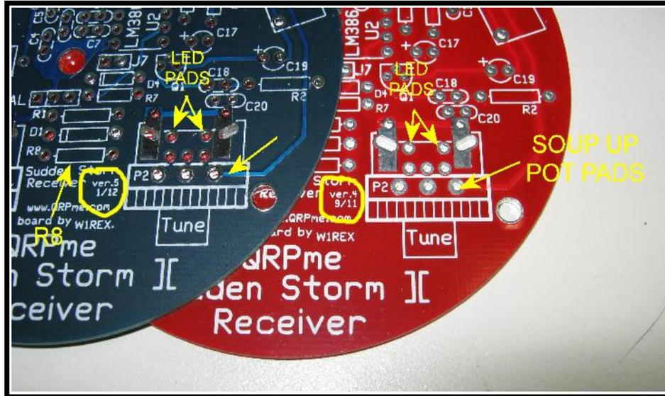
In the lower right, you will find the 2 Soup-up Pot LEDs and the resistor R8. The right side of D6 (Tune Pot LED) is connected to the +9v where it comes 'down' the pcb to feed the Tune pot. The left side of D6 goes thru R8 then on to D5 (Gain Pot LED). The left side of D5 goes to the ground plane.
