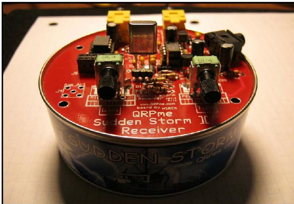
Sudden Storm with standard issue pots installed in the rear (narrow) pot pads. The LEDs and R8 are not installed when using the standard pots.
