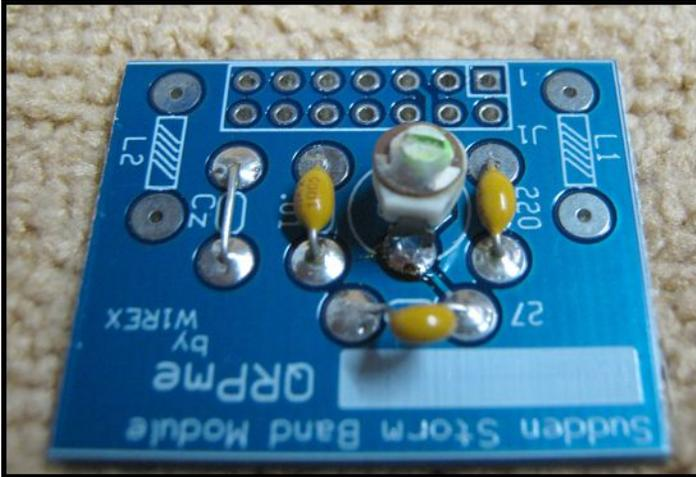
Band module board with caps installed.
