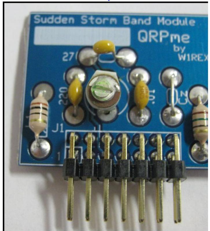
View of completed 40m band module board
