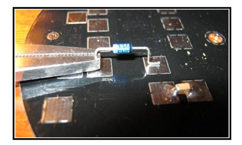
Installing components on Limerick pads is also a cinch using the pliers...
