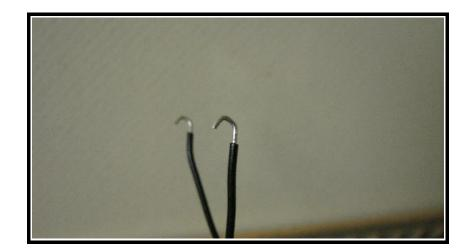
Solder leads to the connectors BEFORE mounting the connectors in the holes in the cans. It is much easier to solder leads to the connectors out in the open than when you have to do it down inside the can. Remember that a good electrical connection starts with a good mechanical connection. Form hooks in the pieces of hookup wire and crimp them into the holes on the connector leads whenever possible.
