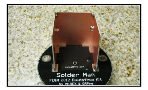
The solder roll holder 'box' is now tack soldered onto the pads on the circuit board.
