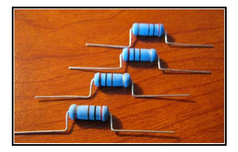
All 4 resistors are mounted onto pads with identical spacing so all the leads are bent alike.
