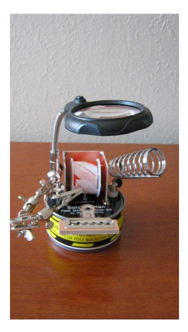
The next step is to punch a couple of holes into the 2 side panels of the solder roll holder. They should be located about 1/4" down from the top edge and a little forward of the center line of the holder. Use either the nail and plastic tubing 'keeper' of the 2 short screws with double nuts to hold your roll of solder in the holder.
