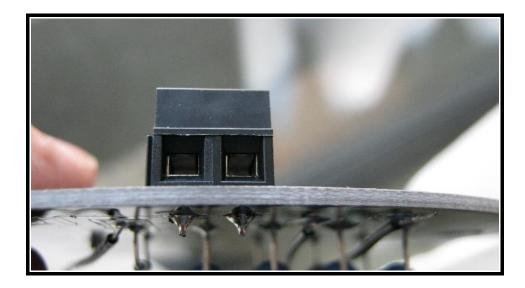
The 2 position screw terminal is soldered to the TOP side of the circuit board.
