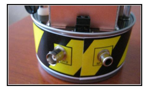
You can solder the 2 connectors in parallel and then use a single set of leads to attach to the proper pads on the circuit board. The Solderman kit is starting to take shape.
