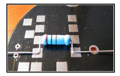
This above picture shows the resistor leads bent in order to stand the resistor up onto the pads for assembly.
