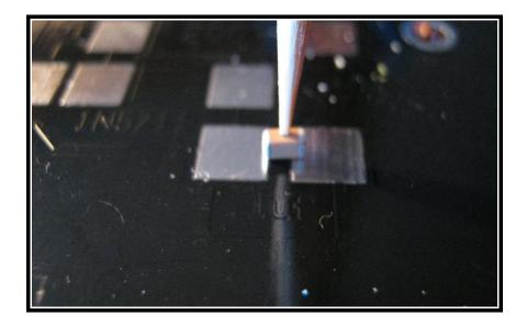
For an additional talking point, the capacitor was chosen as a surface mount component. The component is placed across the corresponding pads (bridging the gap) and held in place using a wooden kitchen skewer......
