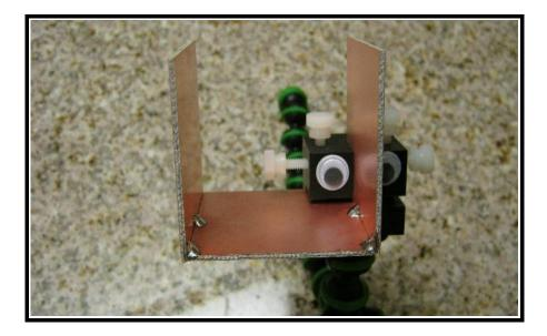
Note the pcb overlap pattern indicated on the circuit board silk screen when soldering the square panels together...
