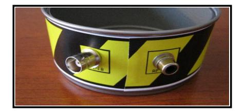
Builders had to apply labels to their cans and then punch 2 appropriate sized holes in the proper locations in the can in order to mount the meter connectors.
