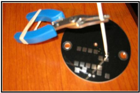
A small pair of pliers with a rubber band around the handles makes a very handy skewer grabber and down pressure device. You can easily re-grip the skewer for each component and also reposition it for ease of assembly. No additional hold down device is needed..just a pair of pliers, a skewer and a rubber band.
