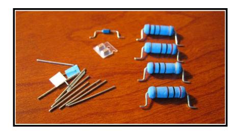
The excess lead length on the 'feet' are cut off so the feet stay on the pads.
