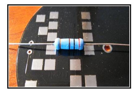
The first step is to prepare the components for soldering onto the board. Here we show the sizing of the 3 watt resistors to determine HOW we need to bend the leads.
