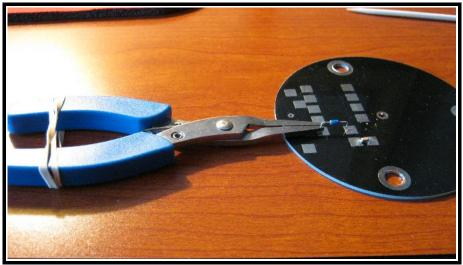
and rubber band trick. The pliers will hold the component vertical while you tack solder the free end using BOTH of you free hands for soldering.
