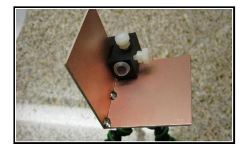
Here is a step designed to gain a little experience building box assemblies out of bare copper circuit board. In the buildathon, we had QRPme's SBSS blocks to hold the panels square while tack soldering. You must allow your tack solder joints to completely cool before removing whatever device you use to hold the joint square or else the cooling solder will 'pull' the joint out from 90 degrees.
