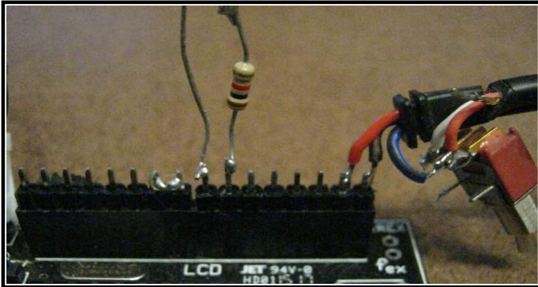
2. INSERT A 8-PIN MALE MOLEX HEADER INTO THE LEFTMOST 8 PINS OF THE LCD HEADER SOCKET. SOLDER A SHORT ACROSS THE RIGHTMOST PINS OF THE MAKE HEADER. THE SHORT IS WHAT TELLS THE MICRO THAT YOU WANT IT TO OPERATE IN THE SERIAL OUTPUT MODE.
