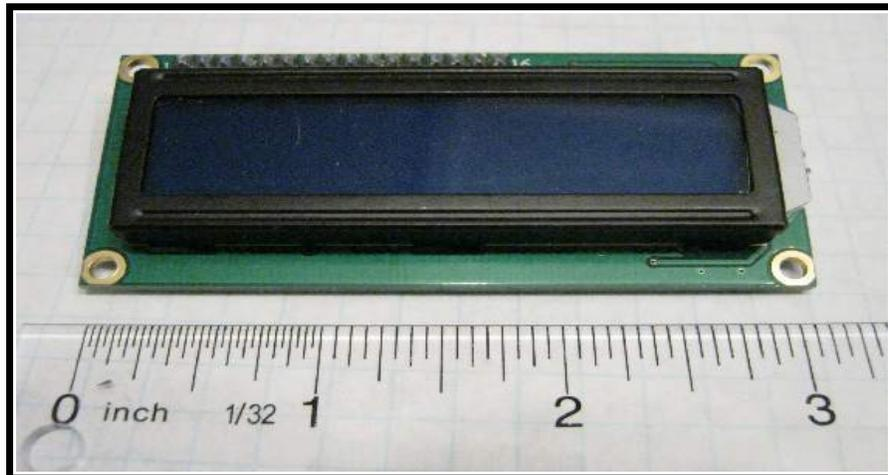
A COMPATIBLE LCD SCREEN IS ABOUT 3" LONG AND USES THE KS0066U OR EQUIVALENT CONTROLLER. IT HAS A 16 PIN INLINE MALE HEADER FOR PLUGGING INTO THE PCB. I USE A GDM1602K LCD MODULE FROM SPARKFUN.
