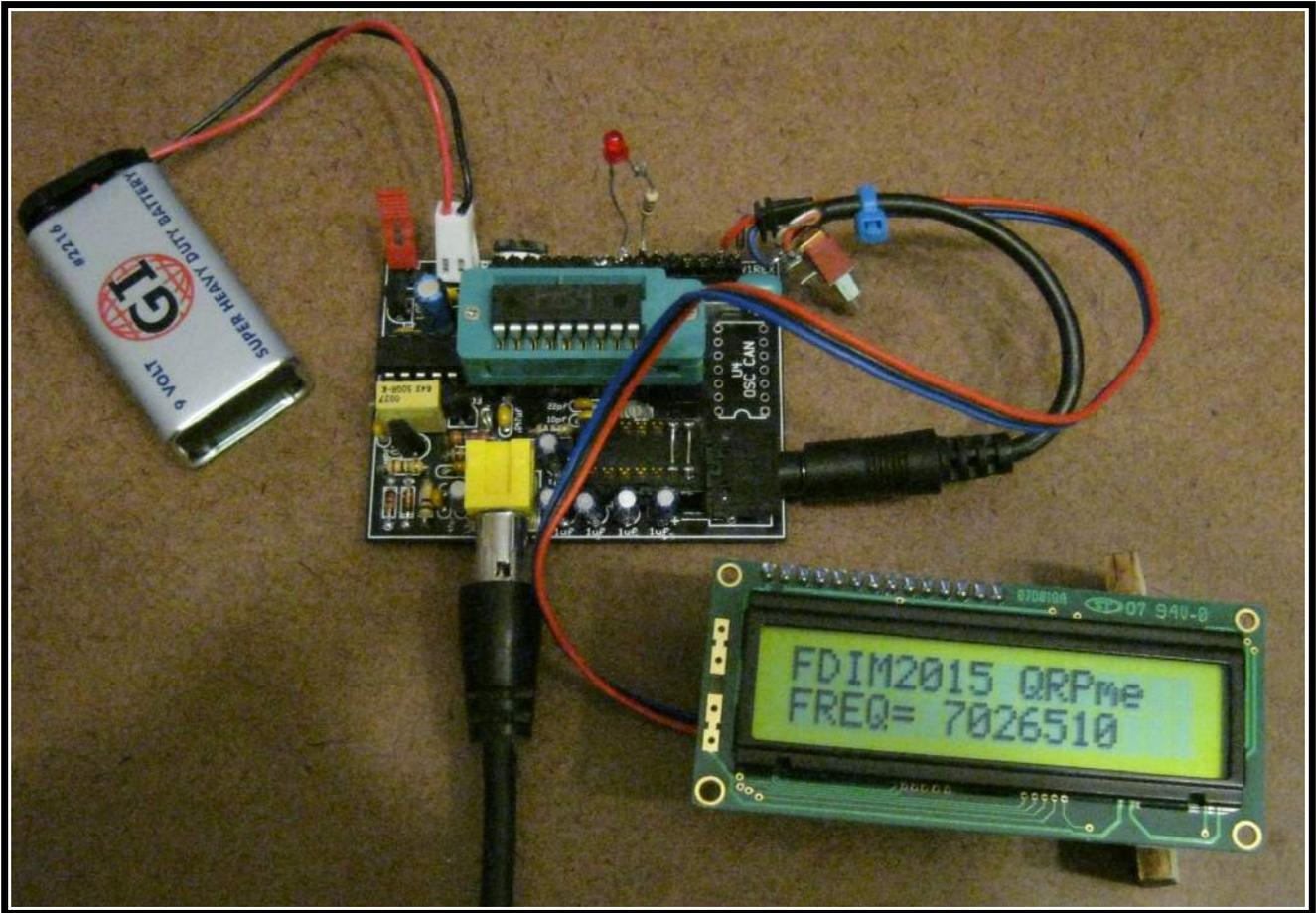
SO HERE IS A COMPLETE SERIAL OUTPUT SETUP SENDING THE FREQUENCY DATA OUT TO A SCOTT EDWARDS SERIAL BACKPACK LCD MODULE.
