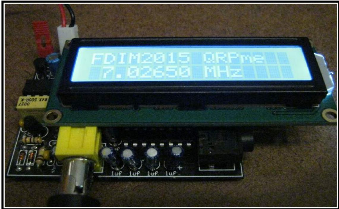
SIMPLY PLUG IN A COMPATIBLE LCD SCREEN AND THE MICRO WILL AUTOMATICALLY SWITCH TO LCD MODE.
