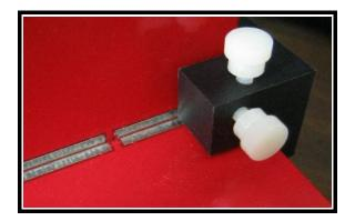
It's intended purpose is to hold PCB stock at right angles while soldering...here is a single SBSS holding two 'Limerick Construction' case panels at a right angle for soldering...
