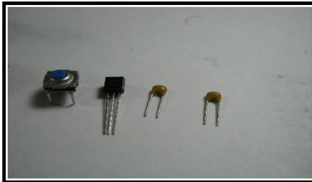
**Select a tactile switch, LM78L05 and two .1uf (104) caps.**
