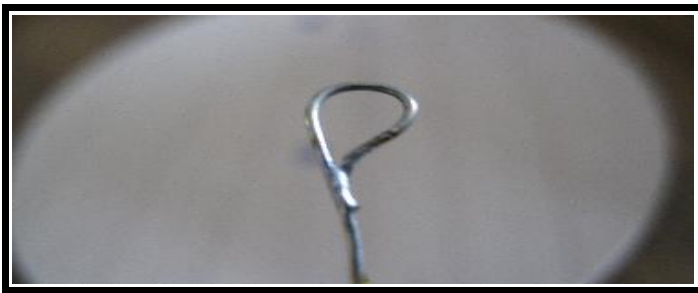
Little clip leads formed from the leftover leads of the resistor.
