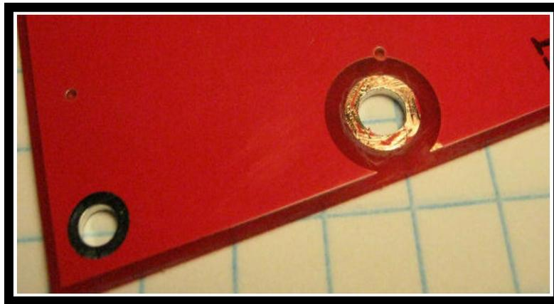
Once you have the 3 larger mounting holes have been scraped, it is now time to prepare the components for mounting Limerick style. The leads of each part need to be formed to fit the Limerick construction pads placed on the circuit board for that part. The easiest way to do this is to form the leads for each part BEFORE soldering anything to the printed circuit board.
