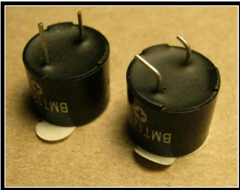
Form the tiny feet on the speaker....making sure the legs are even.
