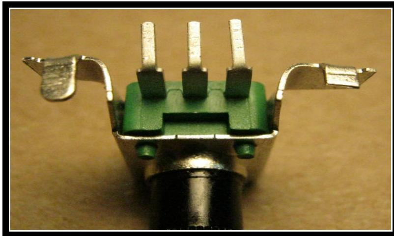
Pot leads bent for Limerick construction
