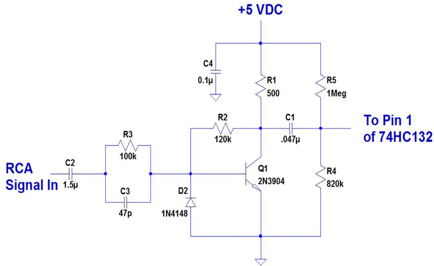
Fig. 4 - X-Checker Signal Conditioner Schematic (After Modifications)
