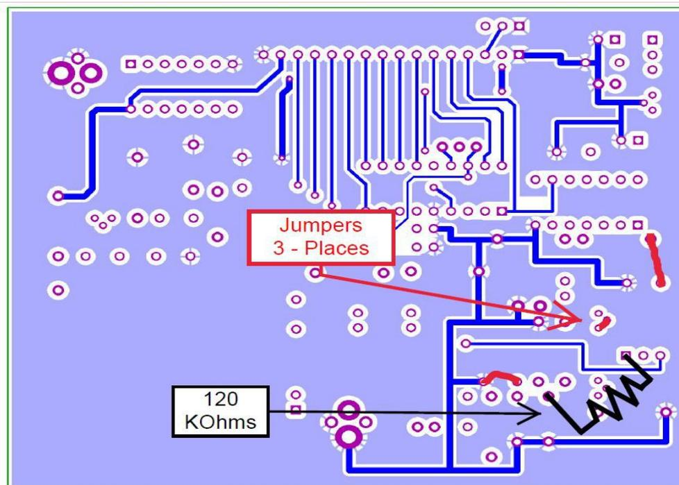
Fig. 3 - X-Checker PCB Solder Side (Bottom) View.
