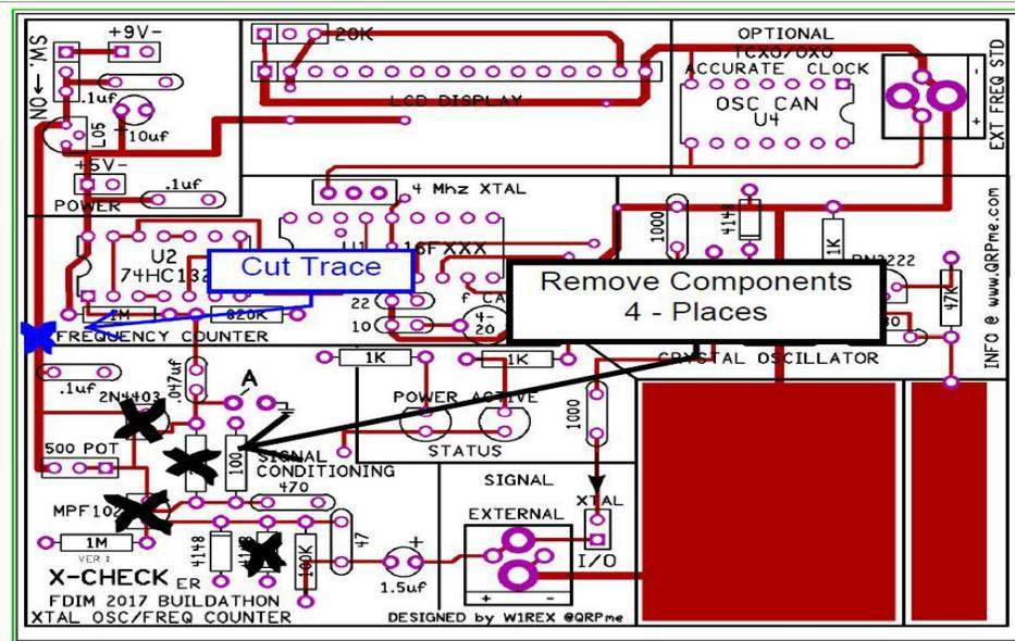
Fig. 2 - X-Checker PCB Component Side (Top) View.
