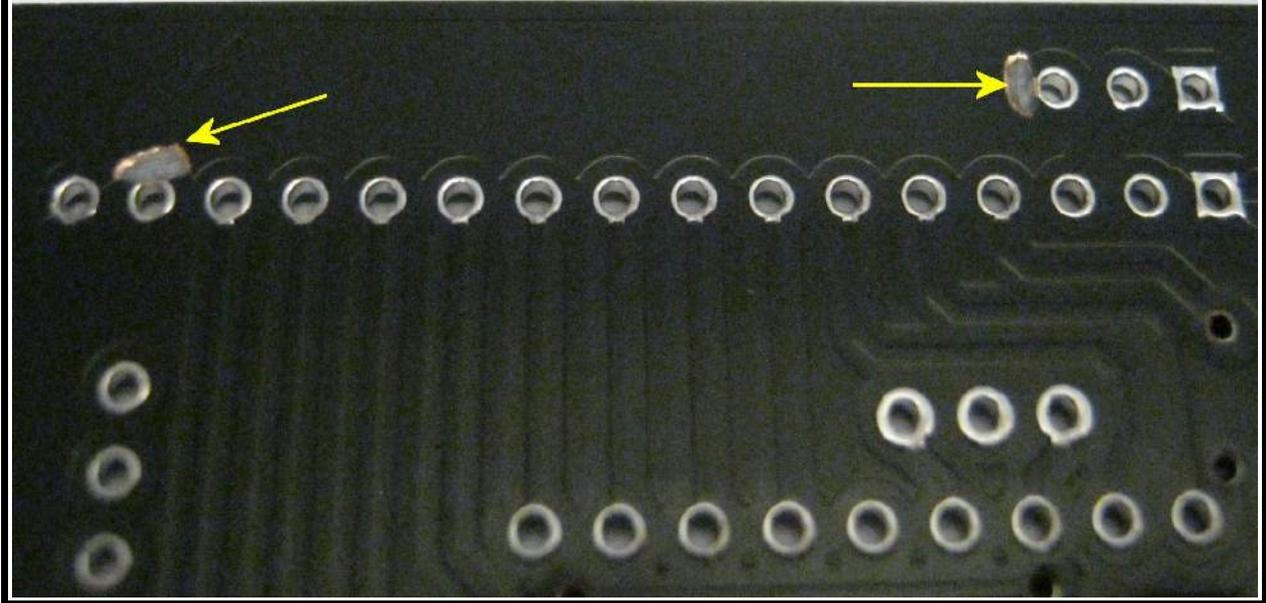
Likewise, the +5 volt power trace from the contrast pot to the LCD backlight pad is shorted to the ground plane on the **BOTTOM** side of the circuit board. Cut the 2 traces just before they enter the ground plane and solder in a short piece of hookup wire to connect the two pads together....after you complete the assembly and the pads have been populated.
