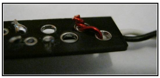
Cut the strain relief off close to the board and bend it flat against the pcb.
