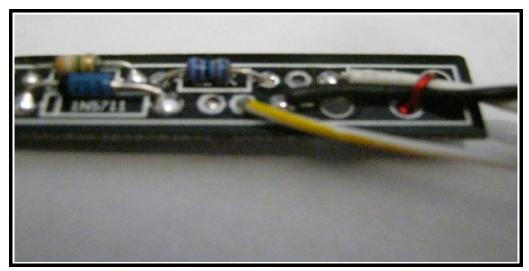
Attach a third wire to one of the 'extra' grounding holes and solder an alligator clip lead to it. This is the grounding wire that you attach to the project you are probing. The twisted pair wires go to the DMM that you are using to read the RF voltages.
