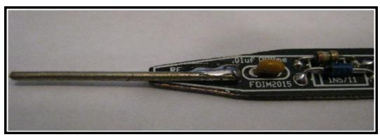
Use a short piece of buss wire to fashion a probe tip. Solder it across BOTH pads on the point of the RF probe pcb.
