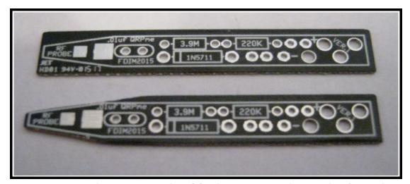
The corners can be snipped off the RF Probe pcb for closer access when using the probe in tight places. Use a pair of tin snips to cut the corners off.
