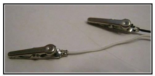
Solder two clip leads onto the other ends of the twisted pair wire. Notice that the wire has been untwisted and that the white (positive) lead is cut (about 1.5 times the length of the alligator clip) longer than the black ground wire.
