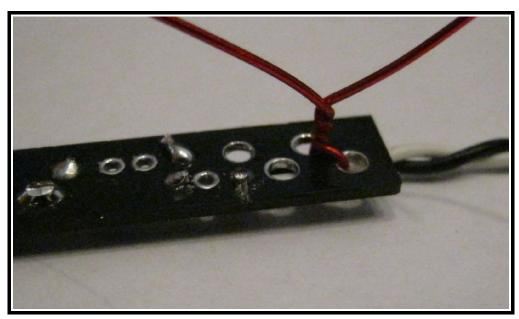
A short piece of magnet wire can be inserted into the larger hole at the end of the pcb and then twisted together to form a strain relief for the twisted pair wires. Don't use solder here as it might melt the insulation on the wires.
