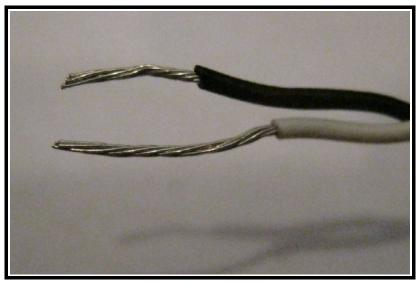
Strip and tin a 1' piece of twisted pair to use as clip leads going to the DMM. Notice that the white positive lead is stripped further back than the black ground lead by about 3/16". This is so that the twisted pair lays flat on the pcb for strain relief purposes. Dry fit your wire before soldering it to make sure it fits nicely at the end of the pcb without bunching or extra wire looping out.
