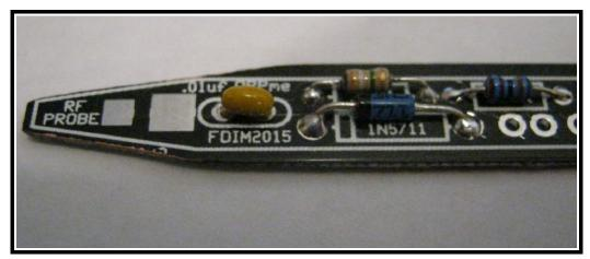
The  $.0\overline{1}$ uf (marked 103) with .1" spacing is next.
