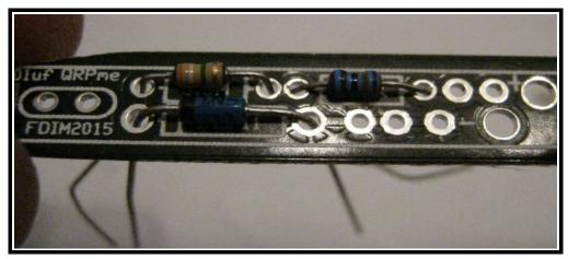
The first 3 parts to install are the 3.9Mohm and 220Kohm resistors and the 1N5711 diode. Glass diodes and 1/8 watt resistors are fragile and could be broken in the bending process when bending without stress relief. Use care, and a nice pair of needle nose pliers to make the lead bends. With nice sharp needles, place the plier tips to the body side of the bend to protest the part from fracturing when making the bend.
