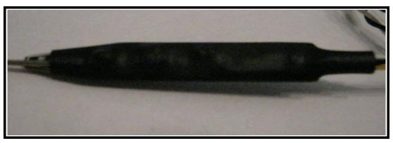
It is not mandatory but you can use heat shrink sleeving to cover the circuitry or install the circuit board into some sort of tube like an old pen or marker body or some plastic item laying about.
