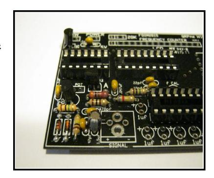
Four 1uf aluminum electrolytic caps are now installed around the MAX232 chip. The polarities change around the 5 caps. Make sure that you get the in right...
