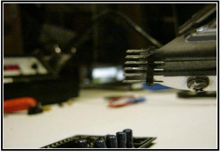
careful deliberate pace as you can see that the pointy tip of the cutter has NO guard. I've used these cutters for several years and have only stabbed my finger holding a part once! That pointy part is VERY POINTY a VERY SHARP and can make a pretty nasty incision into your finger tip VERY quickly! Use SLOW, DELIBERATE, CAREFUL MOTION when approaching your tiny hard electronic part held in you big fleshy soft fingers!!
