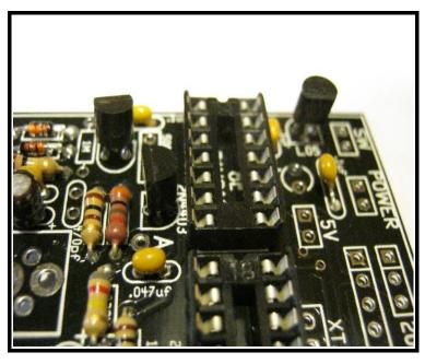
1.5uf installs next to the signal input connector.
