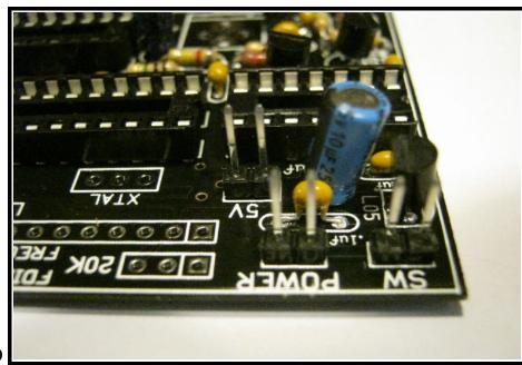
use as a holder or foot when soldering in these headers. I usually hold a single pin with my finger tip and then solder the OTHER pin. When that pin is cool, you solder the pin that I was holding...
