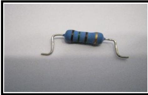
Here is a resistor with the leads bent to fit the pads. Dry fitting the parts before soldering is a must as it is **MUCH** easier to mess with the part while unattached to the board.
