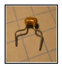
The 2 capacitors are next. You might have to re-bend the caps supplied in your kit to fit the pad spacing. The initial stock of .1uf caps had .2" spacing for .1" spaced pads so it should be re-bent like the left hand picture above. The .22uf cap has .1" spaced leads and needs to be widened for the .2" spaced pads. Bend it like the right hand picture. Install both caps.
