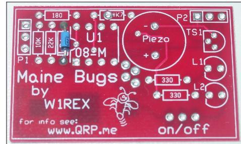
Next install the 6 resistors. Each resistor value is marked on the silkscreen. The two 330 ohm resistors limit the current to the LEDs. They can be replaced by other values based on battery voltage, LED parameters and desired brightness.
