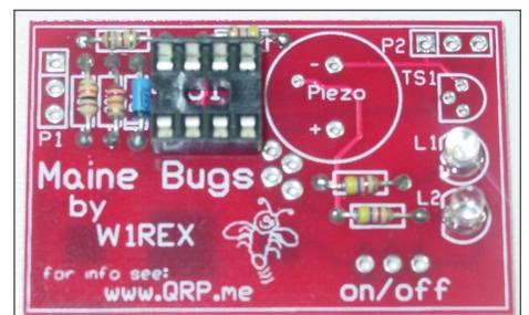
LEDs in a remote location by soldering wires to the LEDs and then soldering the wires to the circuit board at the LED locations.
