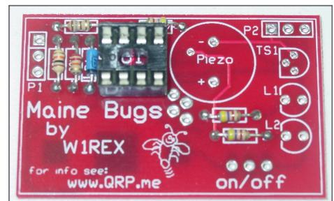
The two LEDs are next. There should be a flattened side on the 'rim' of the LED. Insert the LED so that the LED flat aligns with the silk screen flat. Solder and clip off the excess leads. You could also mount the
