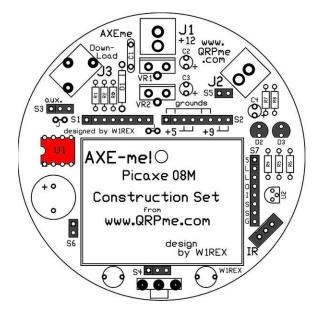
The 8 pin socket is soldered at location U1. Be sure to the socket such that the indentation on the socket matches the indentation on the silk screen. The PICaxe micro should be inserted in the socket AFTER you have finished the entire kit.
