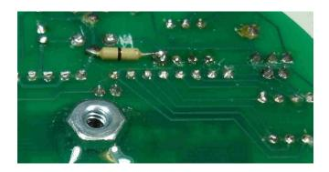
Solder a zero ohm jumper (Black) between the center pin of the L7805 5 volt regulator at VR2 to the bottom pad of diode D1 approximately .4 inches to the right. The trace cut above this mod should already be made.
