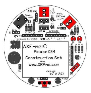
The final 3 parts to be soldered on the board are the 2 RCA jacks at J1 and J2 and the 10K pot at the lower edge of the board. The green LED (clear) can now be inserted into the SIP socket at D2 and the IRLED (blue-ish) at SIP location D3. Likewise, the IR detector can be installed in the SIP connector marked IR with the little black lens pointing out. Pay attention to match up the 'flats' on the LED and the 'flats' on the silk screen.
