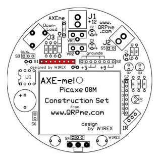
The first items to install are the SIP (single inline package) sockets. There are either 7 or 9 locations on the AXEme board where SIP sockets are installed. You can install the sockets 1 by 1 or all at once. I think it is actually easier to install them all at once using the following method.
