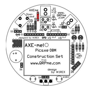
Now install 3 4.7 uF electrolytic capacitors at locations C2, C3 and C4. Make sure that the + lead on the capacitor is inserted in the + hole marked on the silk screen.
