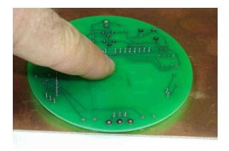
While still applying a little pressure, wiggle the pc board a little bit to help all the SIP sockets settle in and point their little legs straight up... Now you can solder ONE PIN ONLY of each SIP socket to hold it in place.
