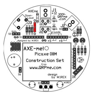
A 1N6263 is installed at location D1. Pay attention to the polarity of the diode. Orient the diode so that the stripe on the diode aligns with the stripe on the silk screen.
