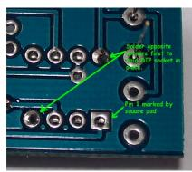
Hold the DIP socket flat with a finger, tack one corner of the socket, tack the opposite corner and then proceed to solder each of the other pins. Go back and re-flow the first two solder joints if needed. Solder S1. If you would prefer to use a larger, more convenient switch, this could
