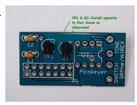
DIP socket and S1 - make sure to line up the notch of the DIP socket with the notch of the silk screen outline (U1) printed on the board. You may wish the dry fit the switch (S1) and the DIP socket to make sure they will fit OK. Once you are happy that they will fit, proceed to solder in place as described next.
