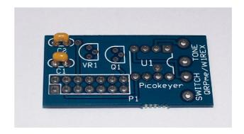
VR1 - 5 volt regulator -Oops! Missteak in the silkscreen on the PCB - install VR1 in the opposite orientation to that shown! VR1 should be marked with something like 78L05, the '05' denoting a regulated 5V output.
